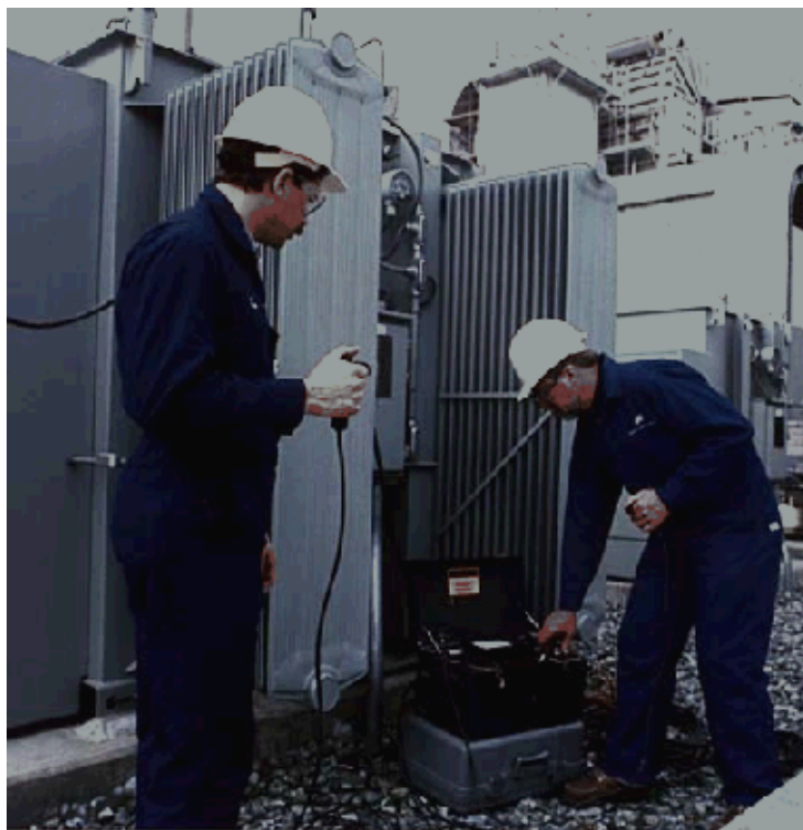
Figure 6-2—Insulation power-factor testing
